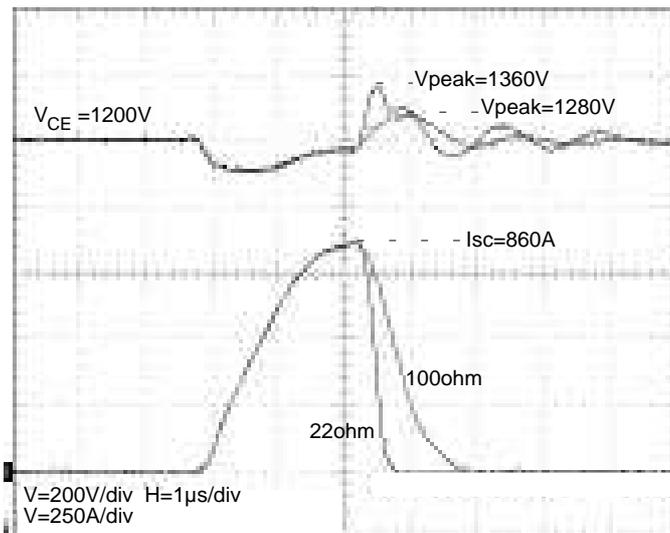
Fig.13 Effect of  $R_{goff-SC}$  in short - circuit
