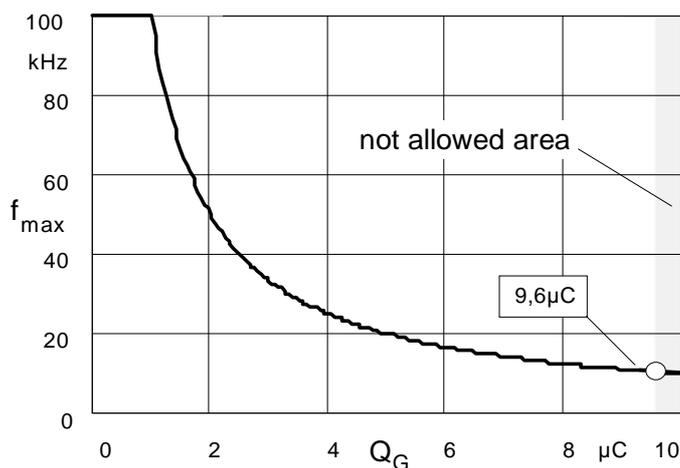
Fig.14 Maximum operating frequency x gate charge
