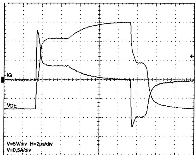
Fig. 11 Output voltage ( $V_{GE}$ ) and output current ( $I_G$ )
